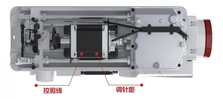
◆ 步进电机控制抬压脚:压脚提升和下降时声音轻柔,压脚高度可调 Stepper motor control to lift the presser foot:
